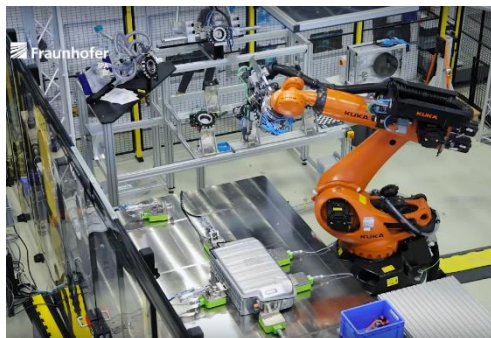
Robot based - Battery disassembly [YouTube-link]
