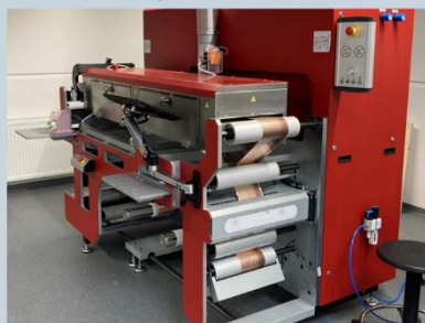
Roll-to-roll coating system for initial feasibility studies (larger pilot-scale systems are available as well)
