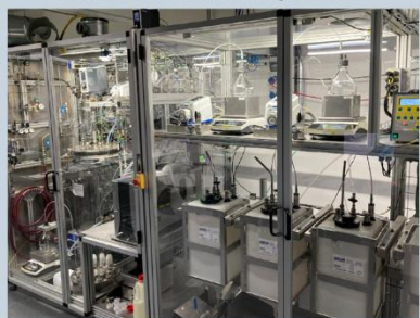
Fully automated synthesis plant for the production of cathode active materials on a kilogram scale
