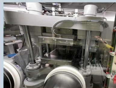
Hot press in glove box for feasibility studies on solid-state batteries (larger systems are available as well)
