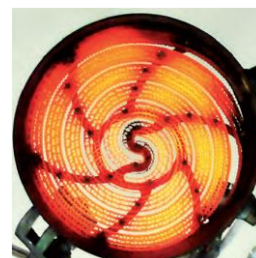
Electrically heated catalyst carrier in development to support thermochemical hydrogen production
