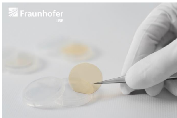
Polished and finished 1-inch AlN Wafer
