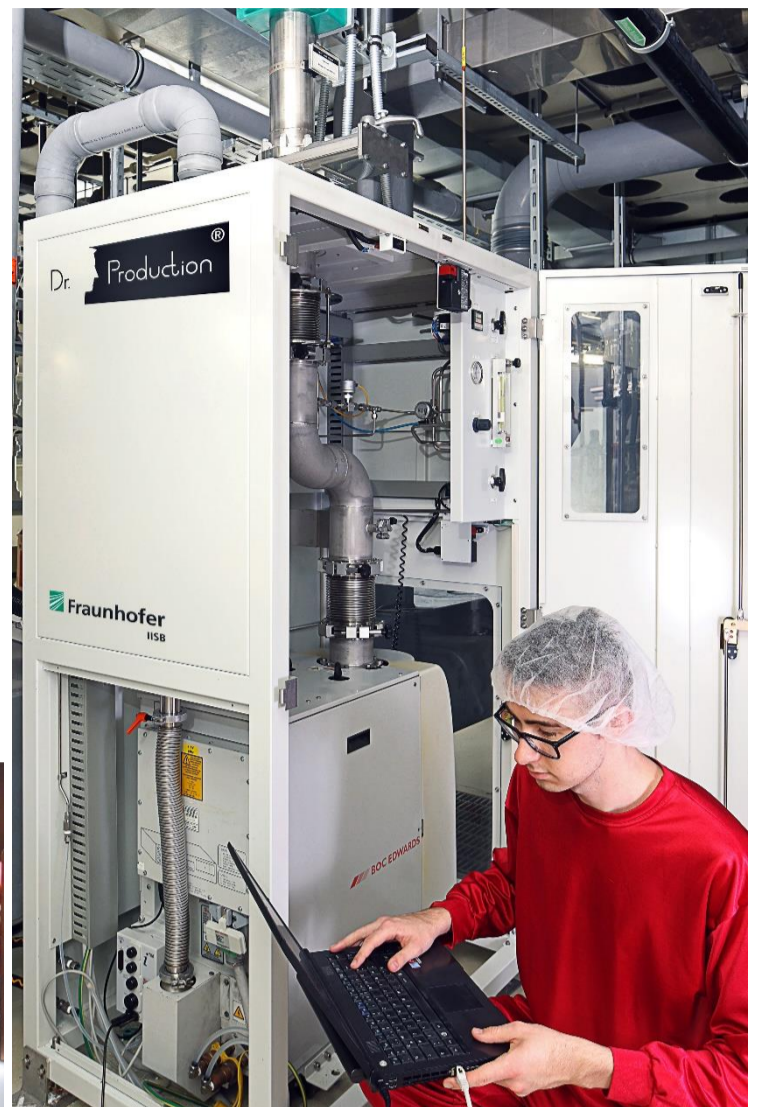
Vacuum system with 100% real-time facility state monitoring for deposition processes in semiconductor manufacturing. A machine-learning algorithm predicts the rest of useful life of the vacuum system until contamination gets critical.
