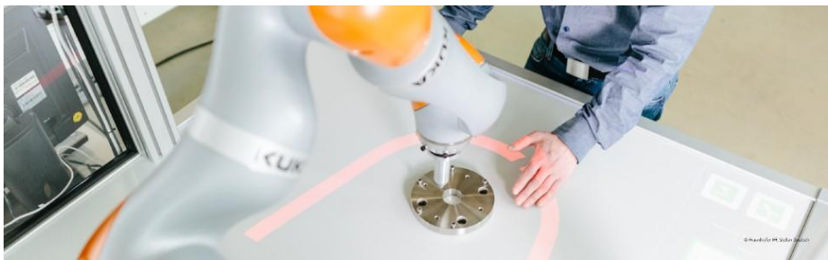
Image 1 – visible light curtains around the workspace as safety lines
