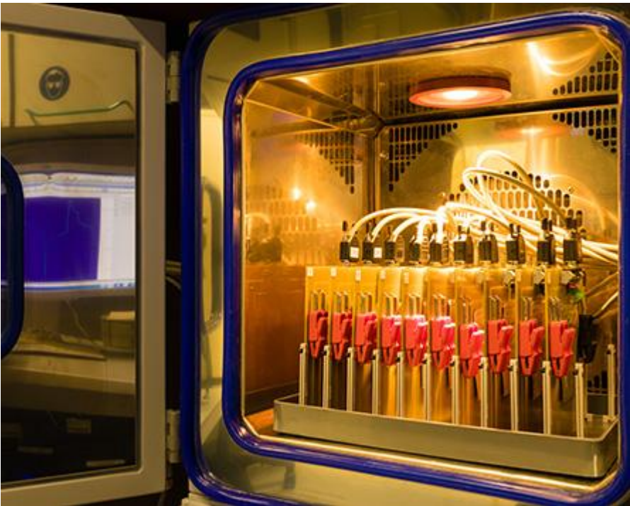
Image 2 – electrochemical characterization of recyclable content, black mass and by-products.
