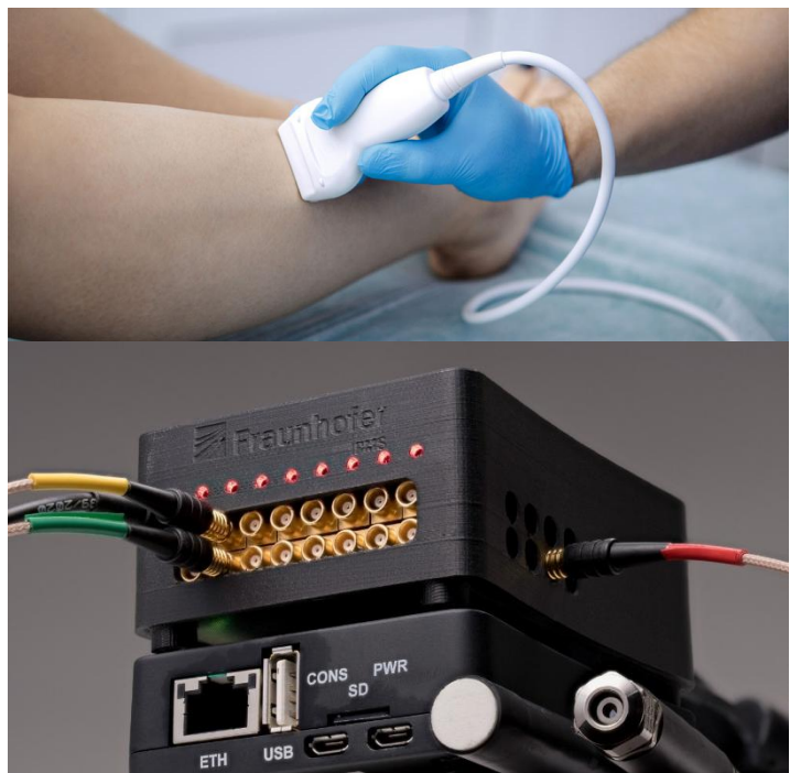
CMUT evaluation kit of Fraunhofer IPMS with a ready-to-use version for testing CMUTs for health application.
