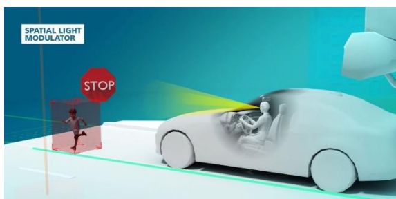
Application example real 3D projection: Automotive Head-Up-Display (HUD)
