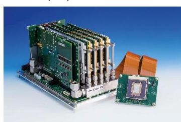
Micromirror array in ceramic package; 512x320 individually addressable mirrors with 48µm pixel size
