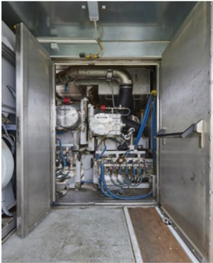
The truck-based mobile system can treat 25 tons of seed per hour. © Fraunhofer/Piotr Banczerowski
