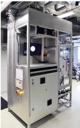
Direct reduction plant on a laboratory scale for reaction kinetic investigations and shaft furnace modeling
